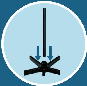
**Step 1:** Insert the black pole into the top of the base with the portion containing the black screw on top.
